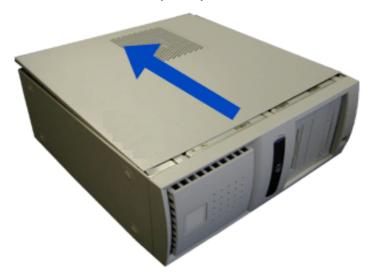
Figure 4 - 3 : Removing the Right Side Door
